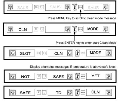
To exit Clean Mode, press the MENU key to display the Clean Mode message. Press ENTER to exit the Clean Mode and return to normal operation. The slot will alternately display SLOT TEMP LOW and the product selection until the temperature is within normal operating limits. If the ENTER key is not pressed within 5 seconds, the slot will return to the Clean Mode.
