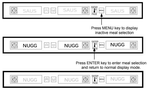
**NOTE:** Active timers will not change to the new meal selection until the timer(s) are stopped or timed out and reset. Active timer(s) are stopped by pressing the timer key. The default menu at start up is for breakfast items.
